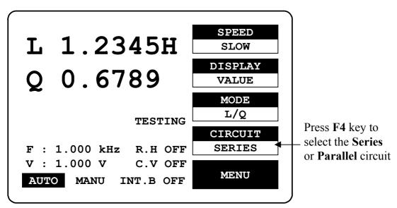
Figure 4-4. Selections of Series & Parallel Circuit
