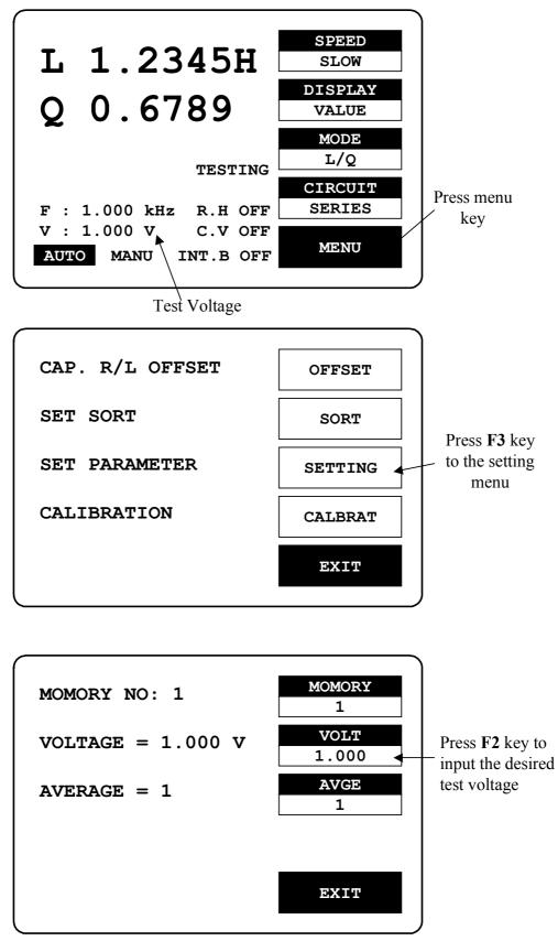
Figure 4-10. Programming of test voltage.
